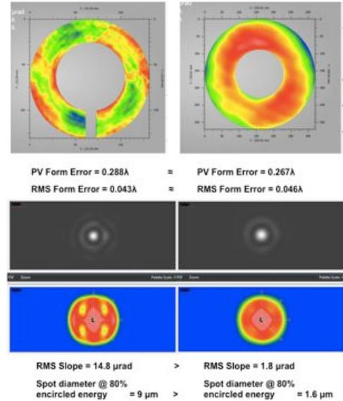
*AOS's aspheric manufacturing process results in low mid-spatial ripples and gradients – which minimizes spot size and maximizes image resolution*
