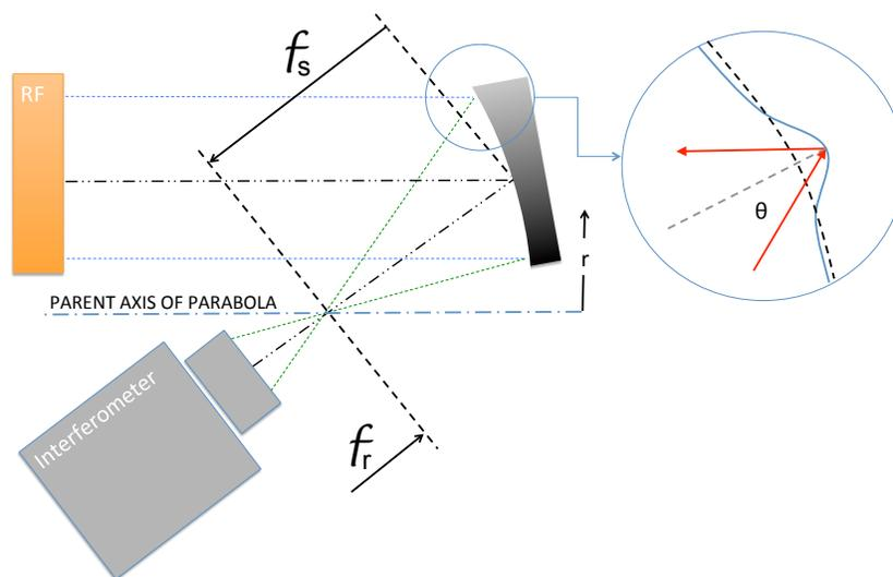
figure 2: Relationship between wavefront error and surface error in an off-axis parabola
