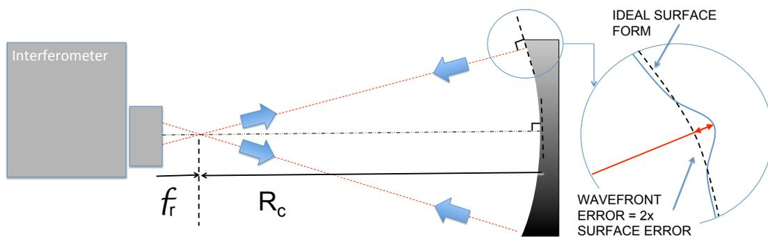
*figure 1: Relationship between wavefront error and surface error in a sphere*
